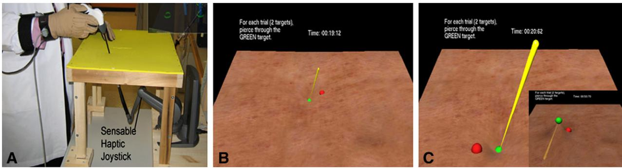
**Fig. 1** A, The user interface, consisting of a laparoscopic instrument connected to a sensible haptic joystick; the user is seen wearing the motion-sensing glove. B, The suturing task in Adult mode, demonstrating the indicated point for needle penetration. C, The suturing task in Pediatric mode. The inset demonstrates bringing the needle back up from the underside of the deformable virtual tissue plane.
