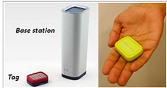
Figure 1. Active RID (SNIFF®) tag and base station
