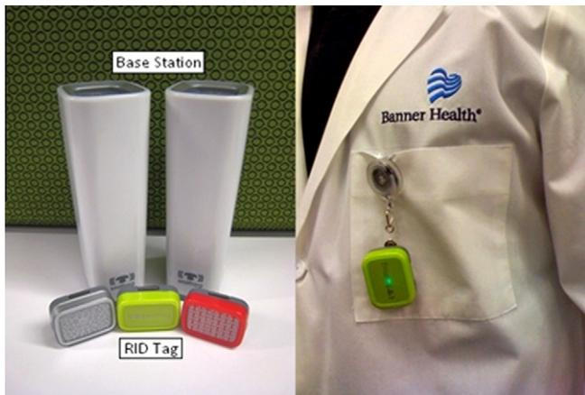
Fig. 3. Active RID (SNiF®) tag and base station.
